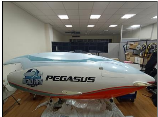
Figure 17 Spray the PU topcoat and use paint protection film
