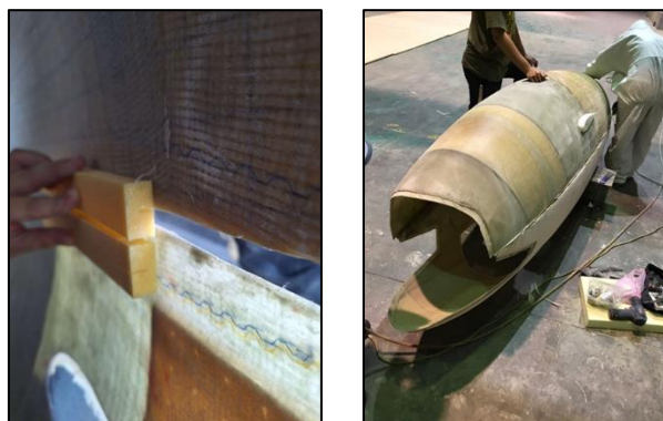
Figure 15 Increase the bonding area
