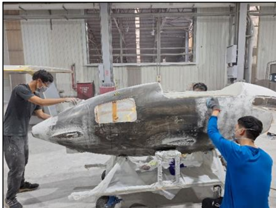
Figure 17 Spray the PU topcoat and use paint protection film
